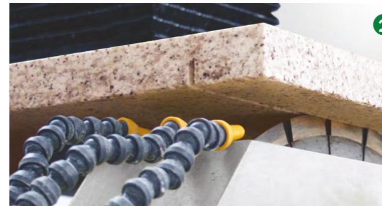
Cutting unit for reinforcement bar complete with disk diameter 400 mm (150 1/8 in) for granite.
